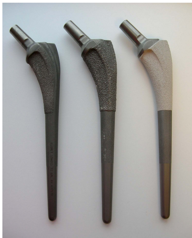
Figure 1 The Mallory-Head Porous femoral component (Biomet, Warsaw, Indiana) is a collarless, titanium, tapered device with plasma-spray coating on the distal third, grit blasted on the middle third, and satin-textured on the proximal third. On the left is shown the component as it was first introduced in August 1984, with the plasma-spray coating covering only 62.5% of the proximal third, on the medial surfaces only. In the middle is shown the standard component with the plasma-spray coating extended circumferentially as a barrier against particulate debris, beginning in January 1987 and as currently available. On the right is shown the component with the option of hydroxyapatite coating applied over the plasma-spray coating on the proximal third, which was first available in November 1988. In addition, a lateralized offset option became available in March 2000.
